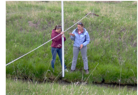
Measuring a stream cross-section
