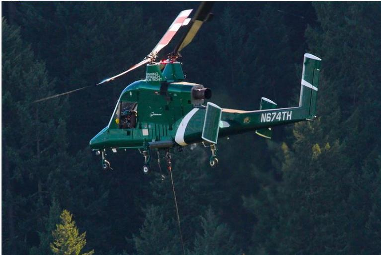
Timberline's K-MAX logging helicopter has two main rotors. They spin in opposite directions, eliminating the need for a tail rotor.
