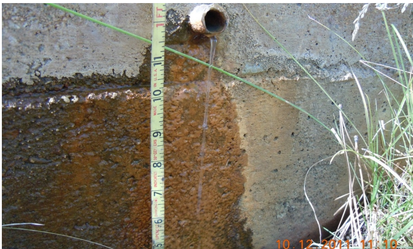
Figure 4. Clover Spring flow as observed on October 12, 2011. Flow rate was estimated at approximately 4 gallons per hour.
