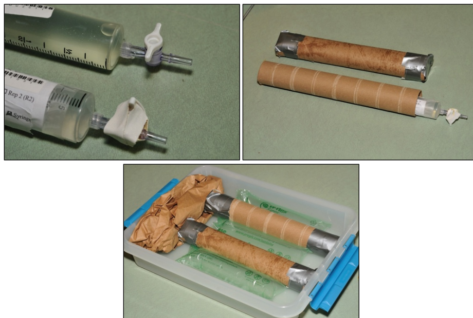
Figure 1–1. Sample syringe packaging for transportation to the lab. Top left: stopcock taped; top right: syringes and packing tubes; bottom: packing tubes packed in a shipping box.
