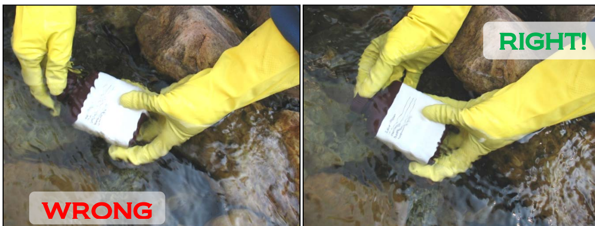
To remove cap under water: DON'T have your hand upstream of the bottle; DO keep your palm UNDER or BESIDE the bottle.
