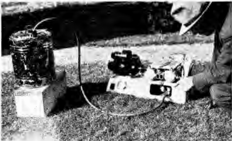
Fuel-feed unit assembled for operation showing flexible-rubber air-pump hose attached to air chuck on carburetor feed line.
