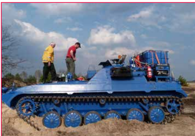
Figure 13—A former BMP OTR-5 command tank is used for safe ignition of prescribed fires on terrain contaminated by unexploded ordnance. The ignition devices include a Pyroshot Green Dragon and a driptorch from an all-terrain vehicle. Photos: Global Fire Monitoring Center.
