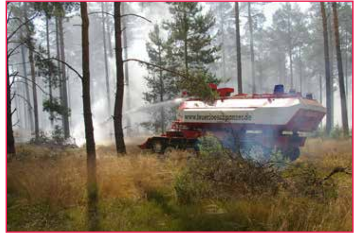
Figure 12—Prescribed fires and wildfires in Brandenburg State (Germany) on terrain contaminated by unexploded ordnance are safely controlled by armored firefighting engines. The SPOT-55 is a converted former T-55 combat tank with high-pressure firefighting equipment and a volume of 11 tons of water or other fire suppressants. Photos: Global Fire Monitoring Center.
