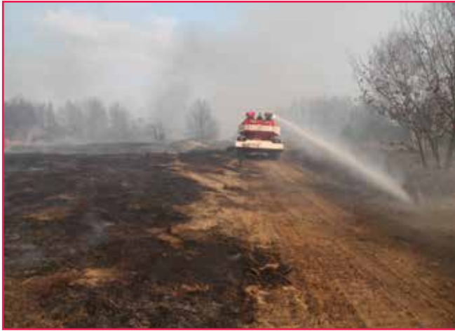
Figure 12—Prescribed fires and wildfires in Brandenburg State (Germany) on terrain contaminated by unexploded ordnance are safely controlled by armored firefighting engines. The SPOT-55 is a converted former T-55 combat tank with high-pressure firefighting equipment and a volume of 11 tons of water or other fire suppressants. Photos: Global Fire Monitoring Center.
