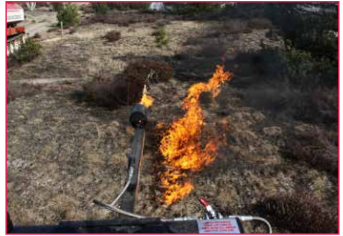
Figure 13—A former BMP OTR-5 command tank is used for safe ignition of prescribed fires on terrain contaminated by unexploded ordnance. The ignition devices include a Pyroshot Green Dragon and a driptorch from an all-terrain vehicle. Photos: Global Fire Monitoring Center.
