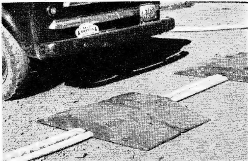
FIGURE 2.—Hose protector in place.
