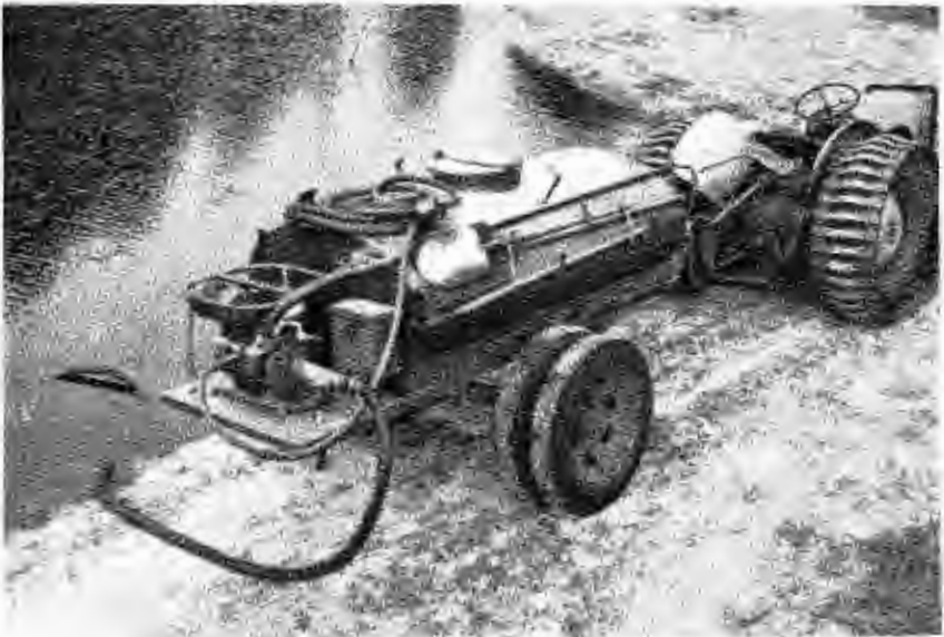
FIGURE 1.—Suppression unit ready for use. At a 10-foot lift the tank can be filled in 7 minutes.
