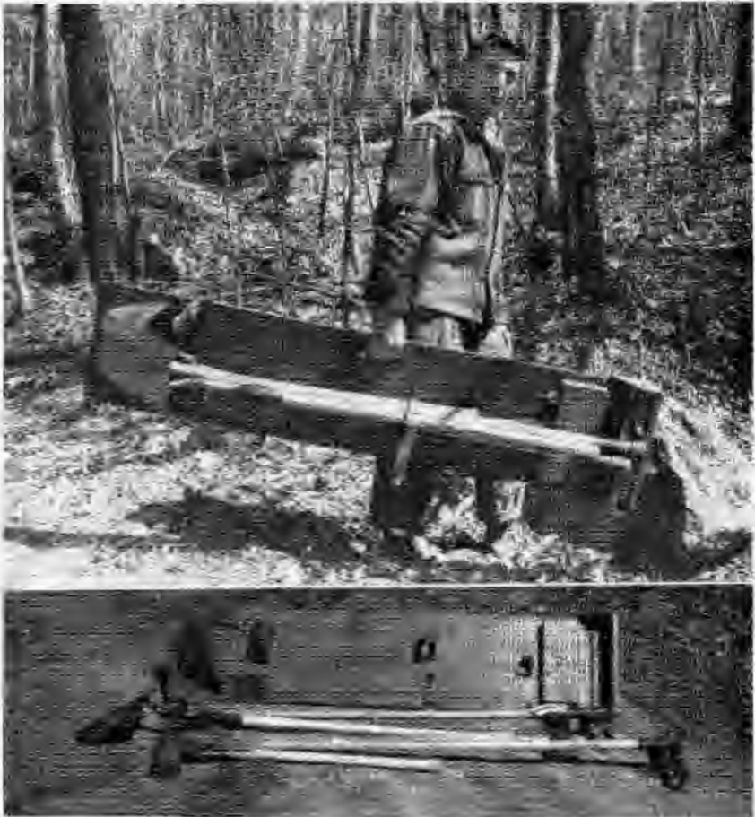
FIGURE 1.—Smokechaser tool unit designed primarily to lie flat in a motor-driven canoe.
