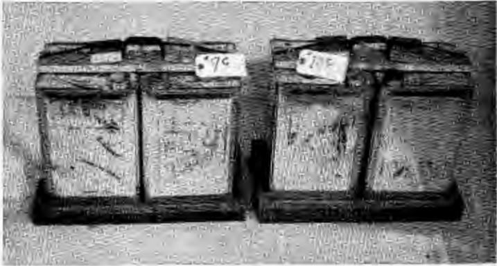
FIGURE 2.—Double can cargo method. Note that board is used to prevent metal band from crushing cans. Small wooden blocks hold cargo handle in place. Honeycomb is 1\frac{1}{2} and 2 inches.
