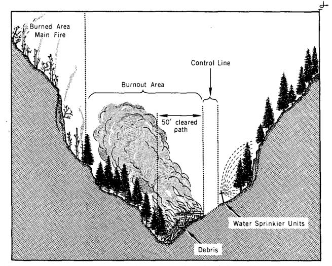
Figure 2.—In this burnout situation, a 20-unit sprinkler system was used to reinfarce the fire control line in the 1967 Eagle Rack Fire. Clearing for a burnout control line resulted in a dense concentration of debris in the canyon bottom. The sprinklers, placed just above the control line, prevented spotting over the line from radiated heat.
