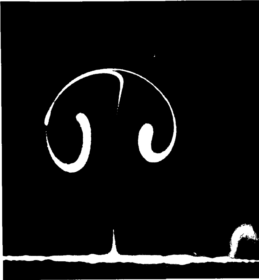
Figure 4 —A laser-illuminated, thin cross section of a vortex pair generated in a wind tunnel over a heated, longitudinally embedded nichrome wire simulating a fire's flank. The photograph was taken with the camera positioned downstream at the tunnel exit directly on the axis of flow.
