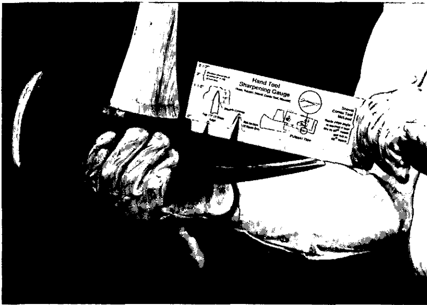
Figure 3 —Gauge is used to check angle of hoe. Photo credit: Missoula Technology and Development Center, Hans Wilbrecht.
