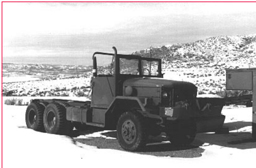
The first step in converting a 6 x 6 water purification van into a wildland fire engine was to remove the van box, which was accomplished in an assembly line at Evanston, WY, in only 2-1/2 hours. Photo: Dana Stone, Wyoming State Forestry, Lyman, WY, 1994.
