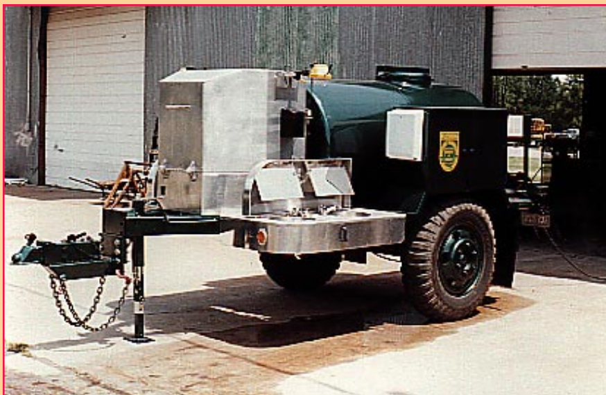
A 400-gallon (1,500-l), fully self-contained portable lavatory unit that will provide hot or cold running water for firefighters and emergency service personnel day or night.
