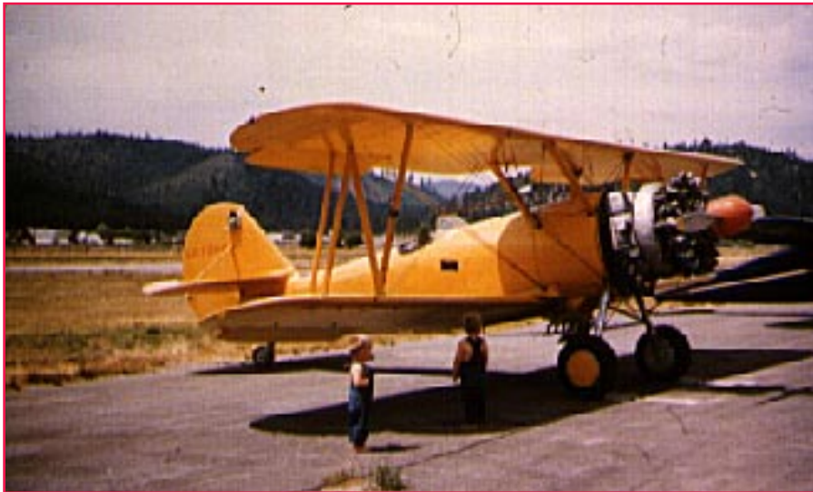
Two children admire an N-3-N airtanker—one of the first types of airplanes the Forest Service ever deployed during California's McKinley Fire in 1956. These small planes can carry 100 to 120 gallons (380 to 450 l) of borate to help suppress the fire. Photo: Courtesy of Lynn R. Biddison, Albuquerque, NM, 1957.
