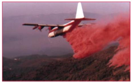
**Figure 1**—*A C–130 dropping retardant on a 1994 wildfire in southern California. C–130's are part of the new generation of large airtankers specified in recommendation 2 of the* National Airtanker Study, *phase 2. Photo: Cecil Stinson, Jr., USDA Forest Service, Shasta-Trinity National Forest, Redding, CA, 1994.*
