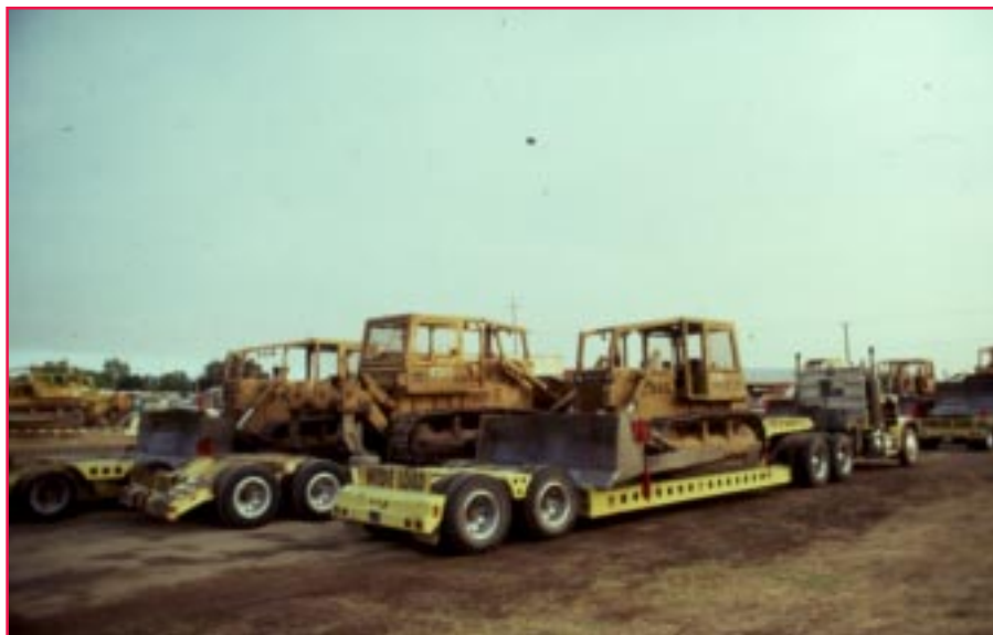
Dozers for wildland firefighting. Engines, dozers, and other contract equipment can drive up costs on wildland fires. Costs can easily exceed $1,000 per day for each piece of contract equipment. Photo: USDA Forest Service, Missoula Technology and Development Center, Missoula, MT.
