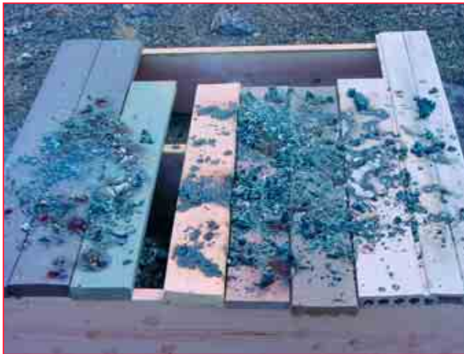
Figure 2—Burning ember test. Hot embers failed to ignite any of the various materials used to build the deck. Photo: Jim Wheeler, Flagstaff Fire Department, Flagstaff, AZ, 2002.
