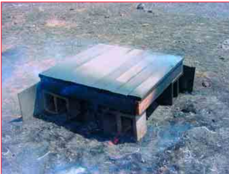
Figure 5— Trex deck test. Trex was difficult to ignite and self-extinguished when the test fire ran out of pine needle surface fuels. Photo: Jim Wheeler, Flagstaff Fire Department, Flagstaff, AZ, 2002.
