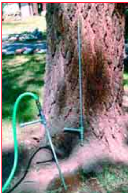
Figure 1—The new mopup nozzle. The nozzle connected to the hose has washed its way 15 inches (38 cm) deep into the hard clay soil around the tree roots. The clay has turned to mud, which can easily be removed with a shovel. The nozzle can also inject class A foam solution into underground areas. Photographer: Bill Gray, San Antonio, TX, 2004.
