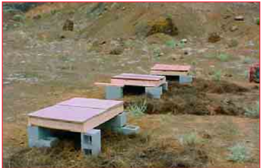
Figure 1—Typical deck test array. Different products were constructed on wooden frames and placed on cement blocks with a simulated fiber-cement stemwall attached. Photo: Jim Wheeler, Flagstaff Fire Department, Flagstaff, AZ, 2002.
