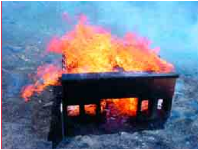
Figure 4— Composite deck test. The test fire easily ignited the composite materials, which burned with high severity. Photo: Jim Wheeler, Flagstaff Fire Department, Flagstaff, AZ, 2002.
