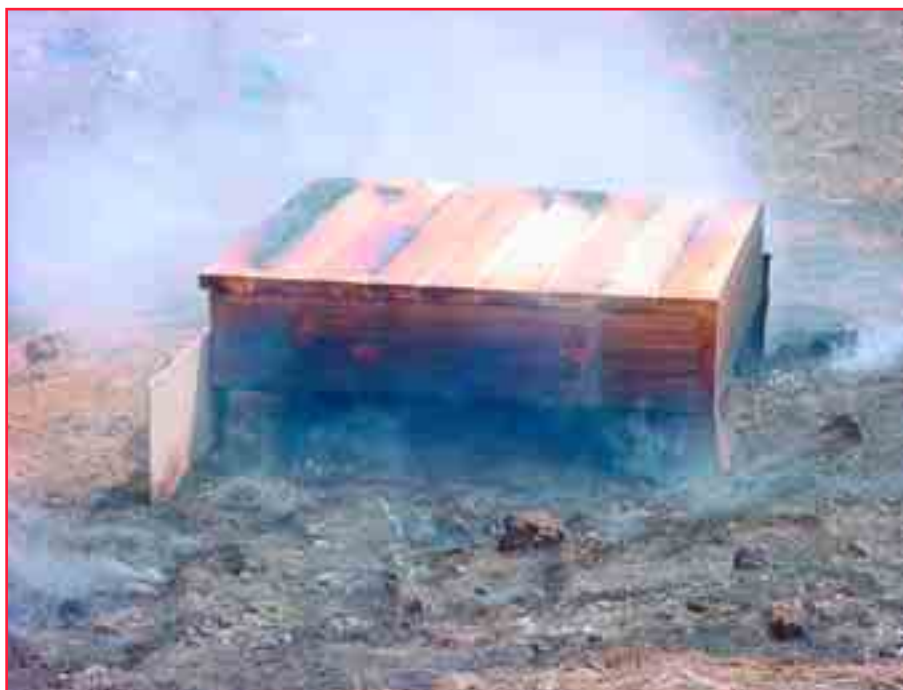
Figure 3—Wood deck test. The wood deck performed well and resisted ignition from the simulated surface fire. However, no stains or varnishes had been applied to its surface before the test. Photo: Jim Wheeler, Flagstaff Fire Department, Flagstaff, AZ, 2002.
