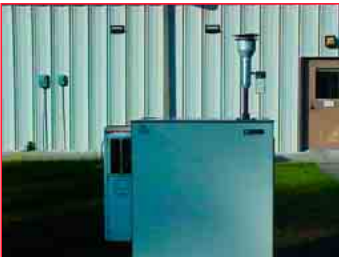
Figure 1—Teom 1400A PM 10 air monitor used on the Apalachicola National Forest, Wakulla Work Center. Photo: Bruce Harvey, USDA Forest Service, Crawfordville, FL, 1996.
