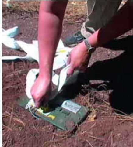
Figure 1 —Testing a buried heat flux sensor during project development on a prescribed burn in California. Photo: Adaptive Management Services Enterprise Team, USDA Forest Service Tahoe National Forest, Nevada City, CA, 2002.
