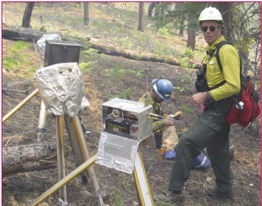
Feel the Heat—Fire-proofed video systems and instrumentation for measuring heat flux, fire behavior, and local weather are installed on the Dragon Complex Wildland Fire Use Incident on the North Rim of the Grand Canyon, AZ, by mechanical engineer Jason Forthofer (sitting) and project leader Colin Hardy. Both men are from the Fire Behavior Research Work Unit, Missoula Fire Sciences Laboratory, Missoula, MT. Photo: Dan Jimenez, Forest Service, Rocky Mountain Research Station, 2005.
