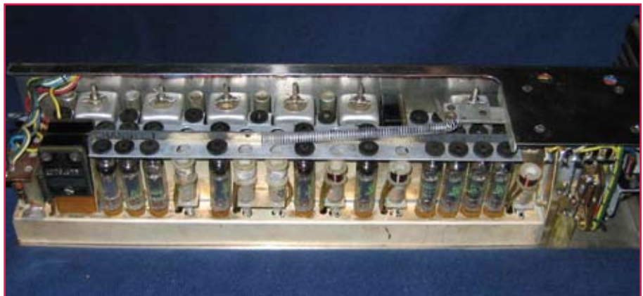
The Forest Service Type SF VHF-FM walkie-talkie, 1947. (Top right) Model A shown with its slide-out battery box. (Top left) Model C with external handset connector. (Below right) Inside the SF, showing its array of 27 tubes and intricate construction. More than 200 radio sets were made before commercial manufacturers began producing their own versions. Photo: Richard Ferranti.
