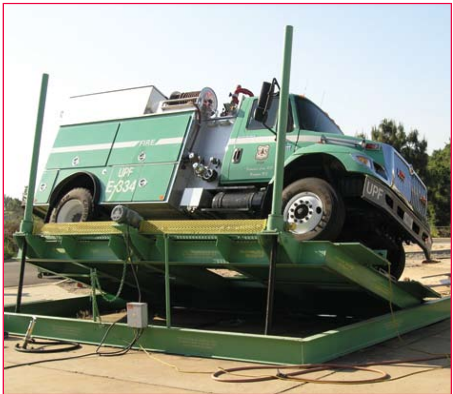
Tilt Table used to conduct Forest Service engine performance evaluations. Photo: SDTDC.
