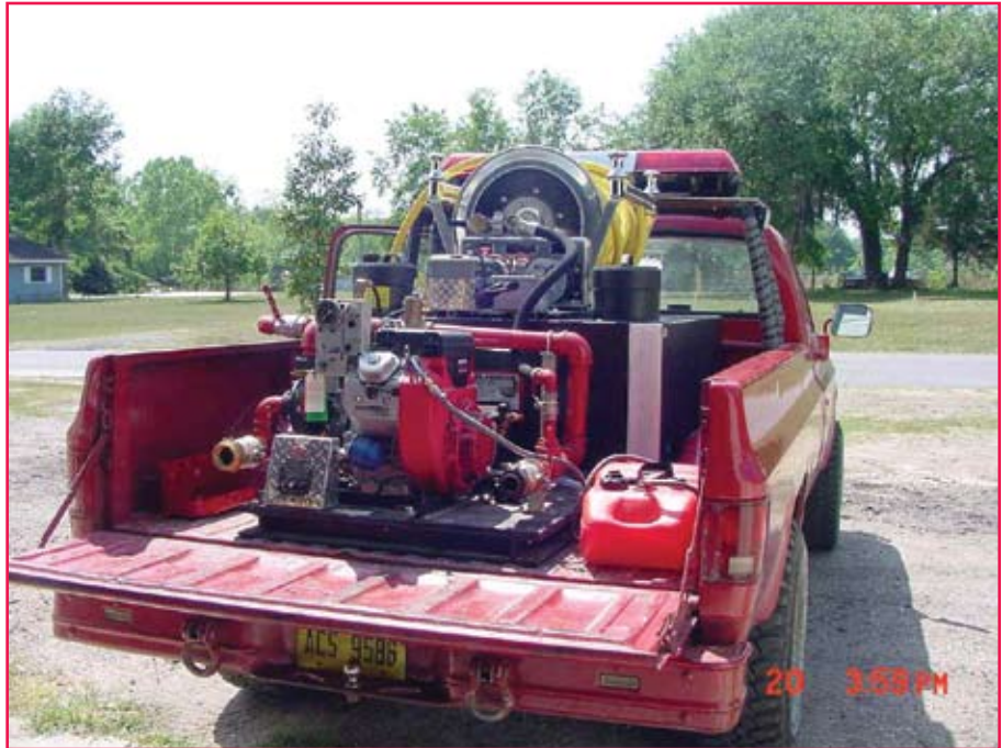
Greenville Volunteer Fire Department, 200-gallon(757-L) skid-mounted unit with foam capability. Photo: Elijah Terrell, Florida Division of Forestry, 2006.
