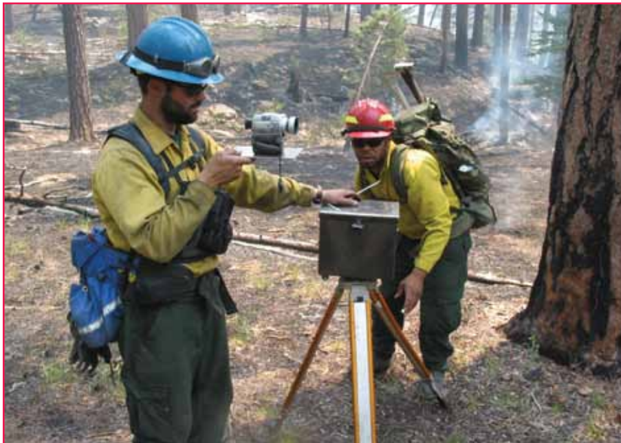
Fire researchers installing a video acquisition box. Photo by Bret Butler, Forest Service.
