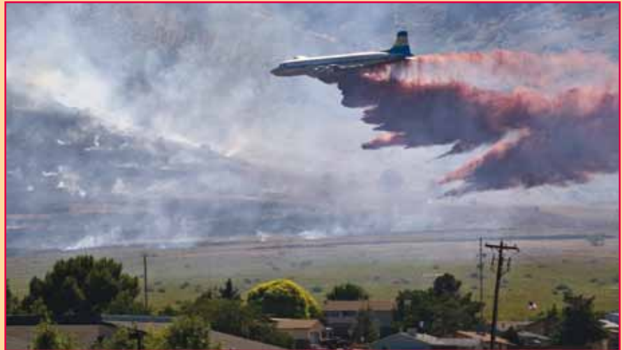
A Douglas DC-7 drops a load of retardant on the Glassford Hill Fire near Prescott Valley, AZ, 2005, to prevent a human-caused fire from spreading toward homes. Photo: Sean Hagan, Dewey, AZ.
