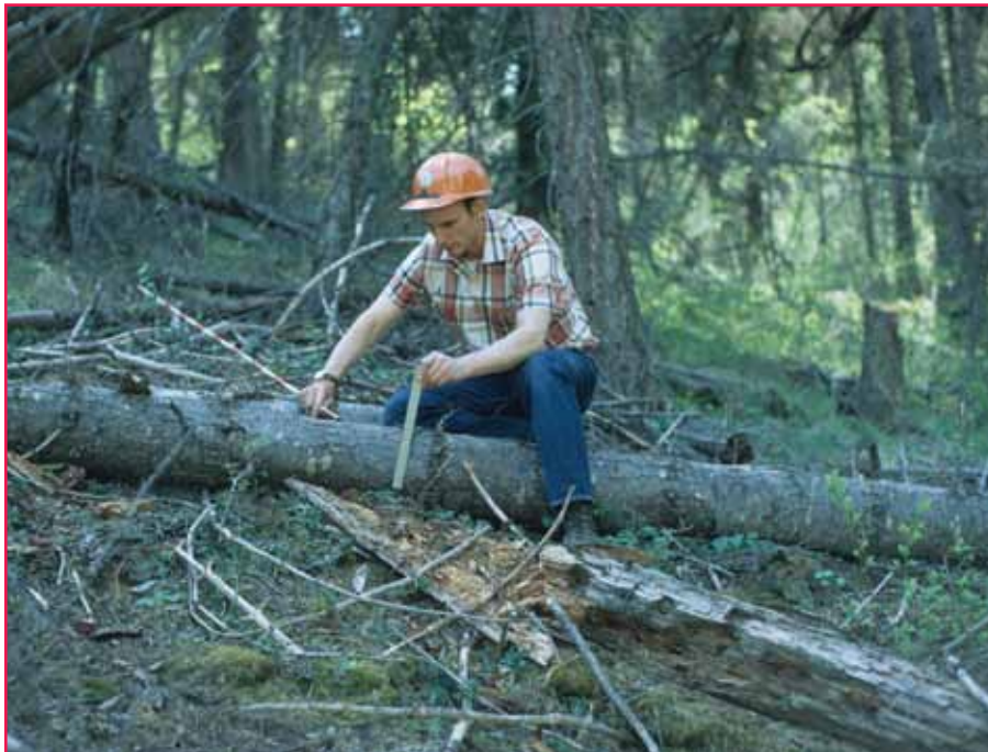
Scientist Jim Brown measures the fuels on the forest floor to establish fuel loading relationships. This 3- by 3-foot (1- by 1-m) area contained about 10 pounds (4.5 kg) of woody fuel. "Brown's transects" remain the standard for fuel load estimation in the field. Photo: Forest Service, 1972.
