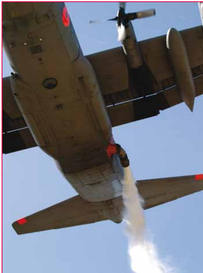
The release nozzle for the MAFFS II is located at the side of the aircraft so that the retardant avoids the turbulence immediately behind the aircraft. Photo: Kari Greer.
