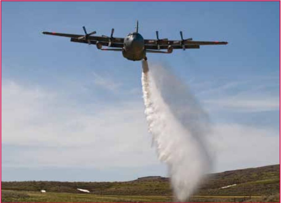
The flexible design of the C-130 allows it to deliver retardant precisely where needed under demanding flying conditions. Here, a C-130 delivers a load of water from a MAFFS II over open ground on a training flight in Idaho. Photo: Kari Greer.
