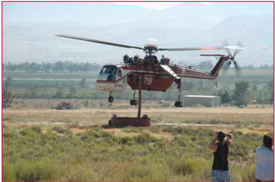
Water tanks were placed to make reloading safe for the equipment involved in operations. Photo: Derrick Davis.
