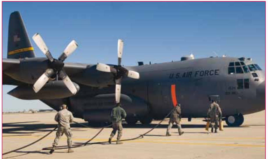
Operation of a MAFFS-equipped C-130 requires numerous specialists, including the loading crew, flight crew, MAFFS crew, and ground control personnel. Here, the crew prepares to load the unit from outside the aircraft during training exercises. Photo: Kari Greer.
