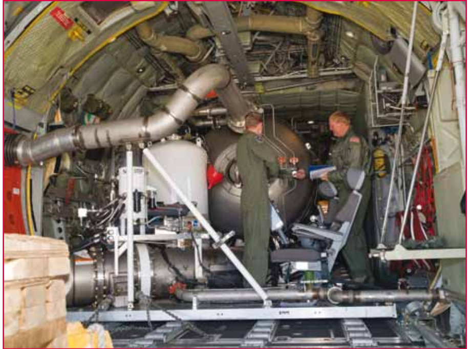
The MAFFS II unit can be rolled into the C-130's cargo bay by way of the loading ramp at the back of the aircraft. In this view, the pipe at the operator's feet running to the right is the retardant intake line, the retardant tank is at the back, the white tank on the left is the foam injection tank, and the large, silver circular tank between the operator and the white foam tank is the pressure vessel. The delivery line is at the lower left, and the air return for the retardant tank is at the upper left. The operator's seat and control console face the delivery line. Photo: Kari Greer.
