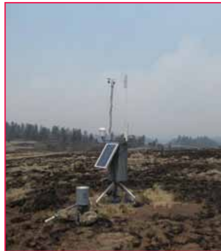
Deployed to a grassy area during the Wallow Fire, AZ, this IRAWS was subjected to a burnover but continued to operate properly. Photo: Alan Hester, BLM, June 2011.
