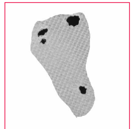
Figure 3.—Trampoline segment inverted and cropped to remove unwanted signatures from trampoline mesh.
