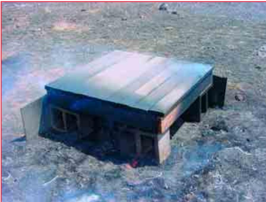
Figure 5—*Trex deck test. Trex was difficult to ignite and self-extinguished when the test fire ran out of pine needle surface fuels. Photo: Jim Wheeler, Flagstaff Fire Department, Flagstaff, AZ, 2002.*
