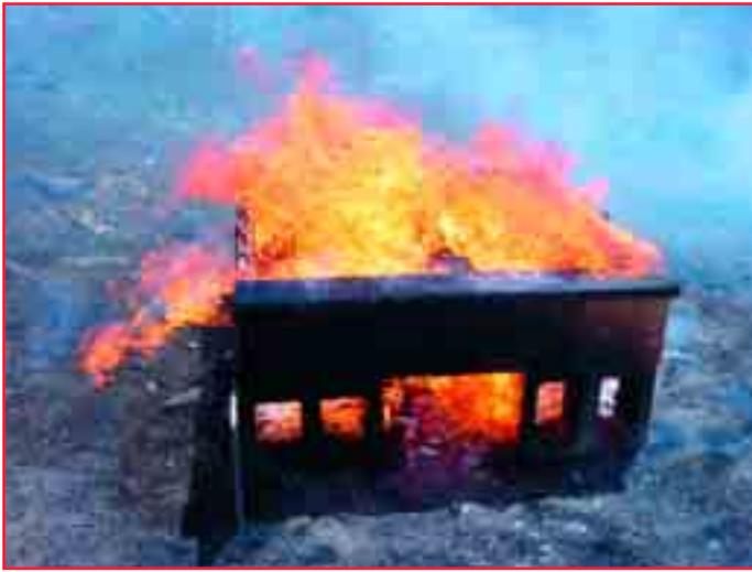
Figure 4—*Composite deck test. The test fire easily ignited the composite materials, which burned with high severity. Photo: Jim Wheeler, Flagstaff Fire Department, Flagstaff, AZ, 2002.*
