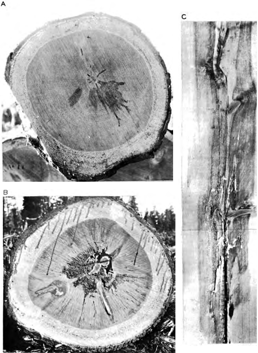
FIGURE 4. —Appearance of red rot: A , Incipient decay showing at the end of a saw log; B , advanced decay showing at the end of a saw log; C , advanced decay bordered by incipient decay in the heartwood of a board—the centrally located area of disintegration probably indicates where rot entered the trunk.
