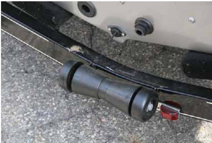
**Figure 10 Trailer Frame & Roller. (note boat drains)**
