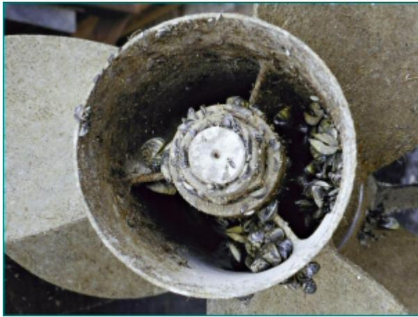
**Figure 18 Mussels Clog Propeller Assembly**
