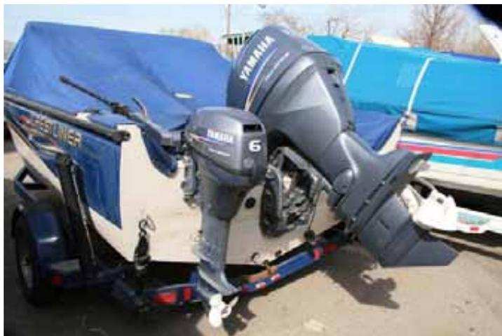
Figure 3 Two Outboard Motors On A Transom
