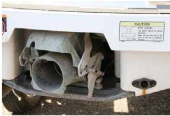
**Figure 41 Personal Watercraft Steering Nozzle (note hull drain)**
