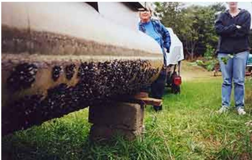
**Figure 39 Pontoon Boat With Mussel Infestation**
