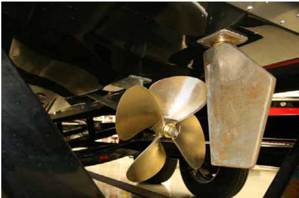
**Figure 5 Inboard Motor Boat With Propeller & Rudder**
