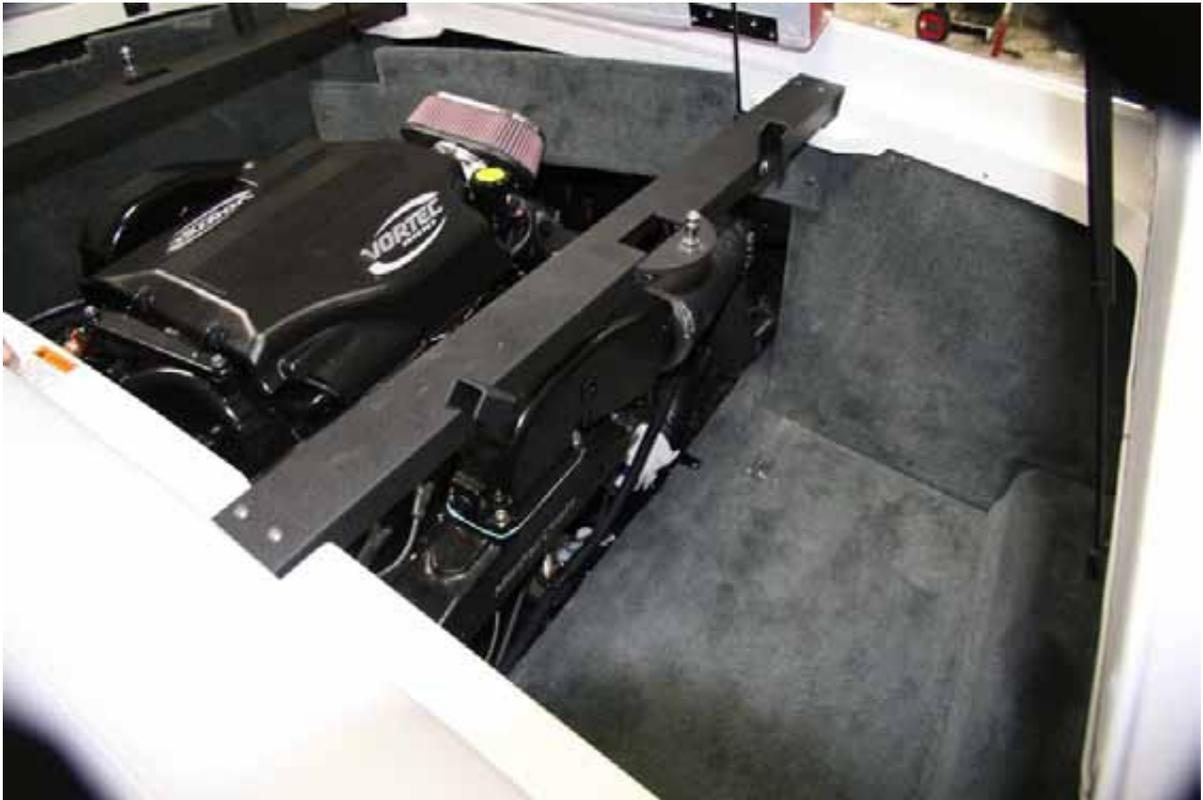
**Figure 25 Water Ski Boat -- Ballast Water Lines Running Alongside Engine (small white caps)**
