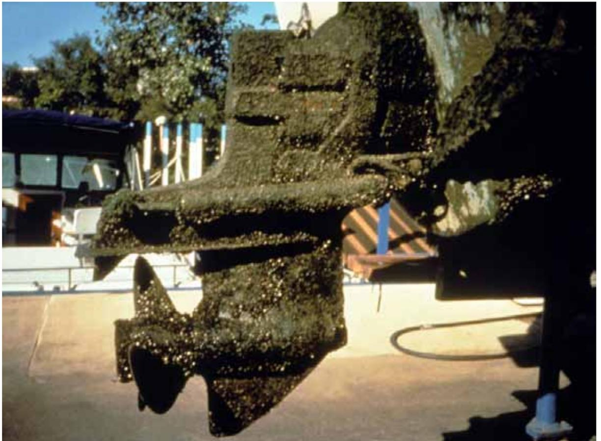
**Figure 20 Thick Mussel Encrustation On Motor & Boat**
