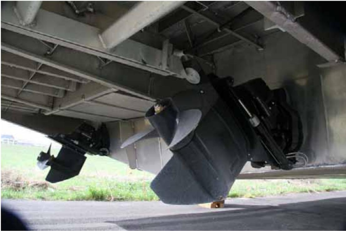
**Figure 31 Houseboat Back End With Motors** (lots of places for mussels to attach & infest, hard to clean)
