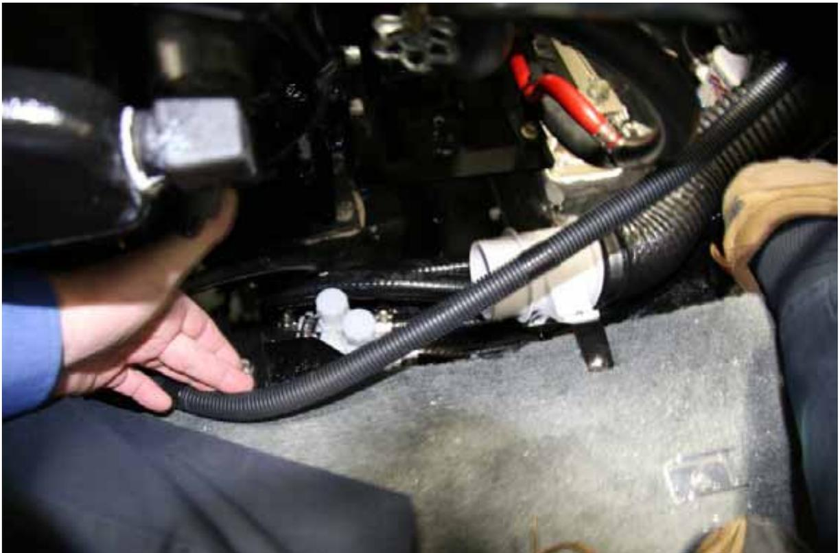
**Figure 26 Ballast System Water Lines - Small White Access Caps (used to introduce mussel-killing solution)**
