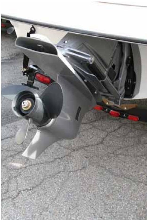
**Figure 4 Stern Drive Motor With Propeller**
