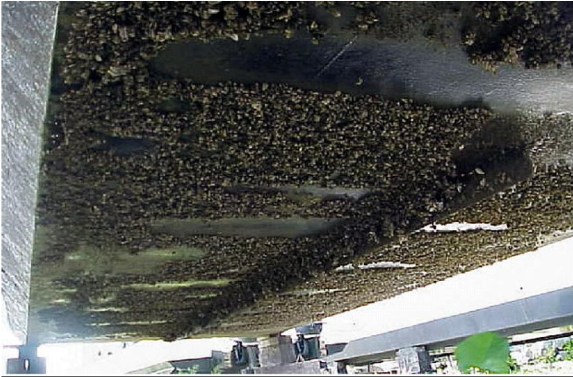
**Figure 35 Flat- Bottom Boat With Mussels** (think houseboat with water intakes)
