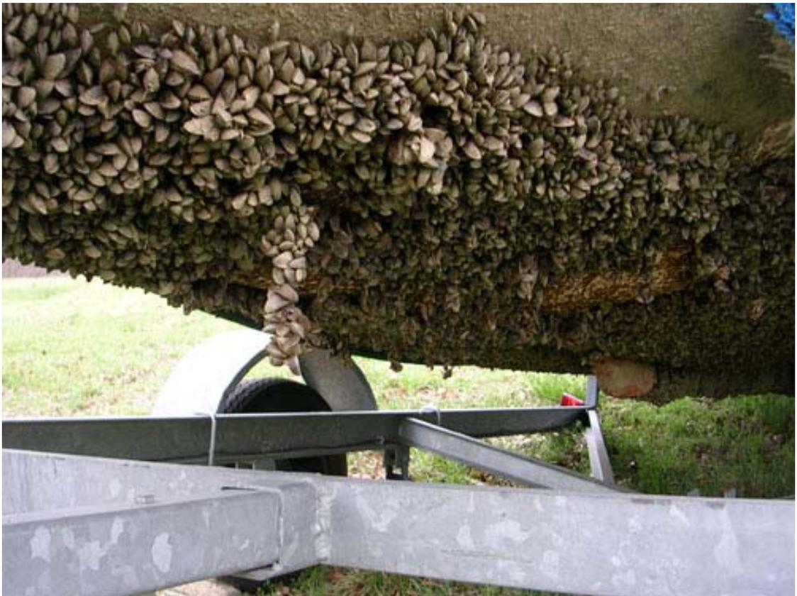
**Figure 36 Seriously Mussel-Encrusted Sailboat Bottom** (note where centerboard would fit)
