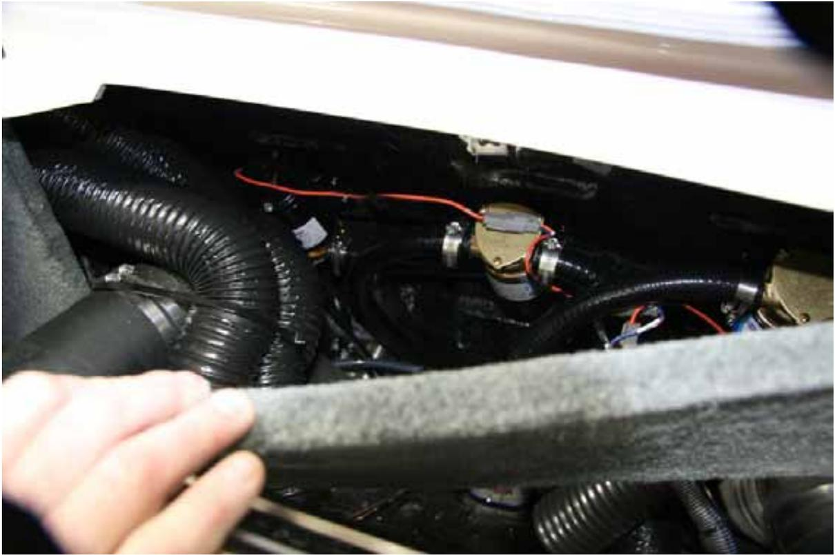
**Figure 27 Ballast System Water Pump**
