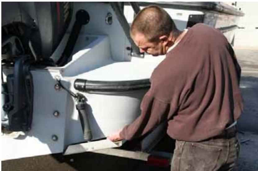
**Figure 8 Carefully Feeling Hull & Trim Tab**
