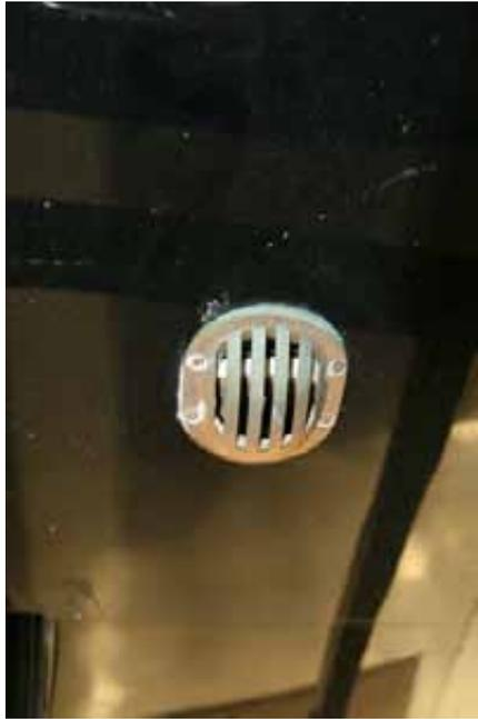
**Figure 12 Water Intake On Hull Under Boat**
