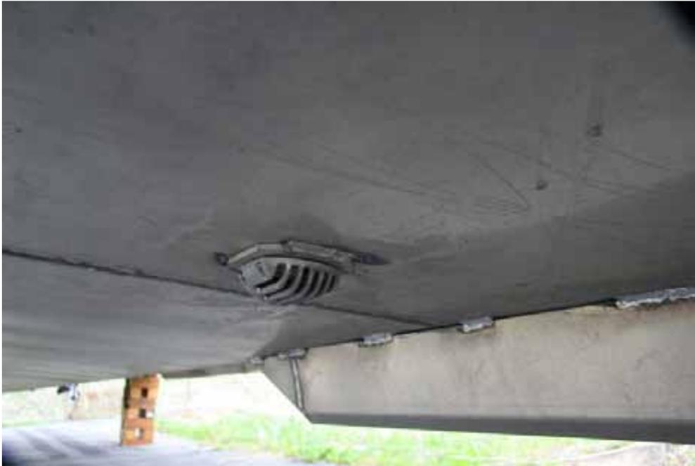
**Figure 33 Underside of Houseboat With Water Intake** (one of several on a typical houseboat)
