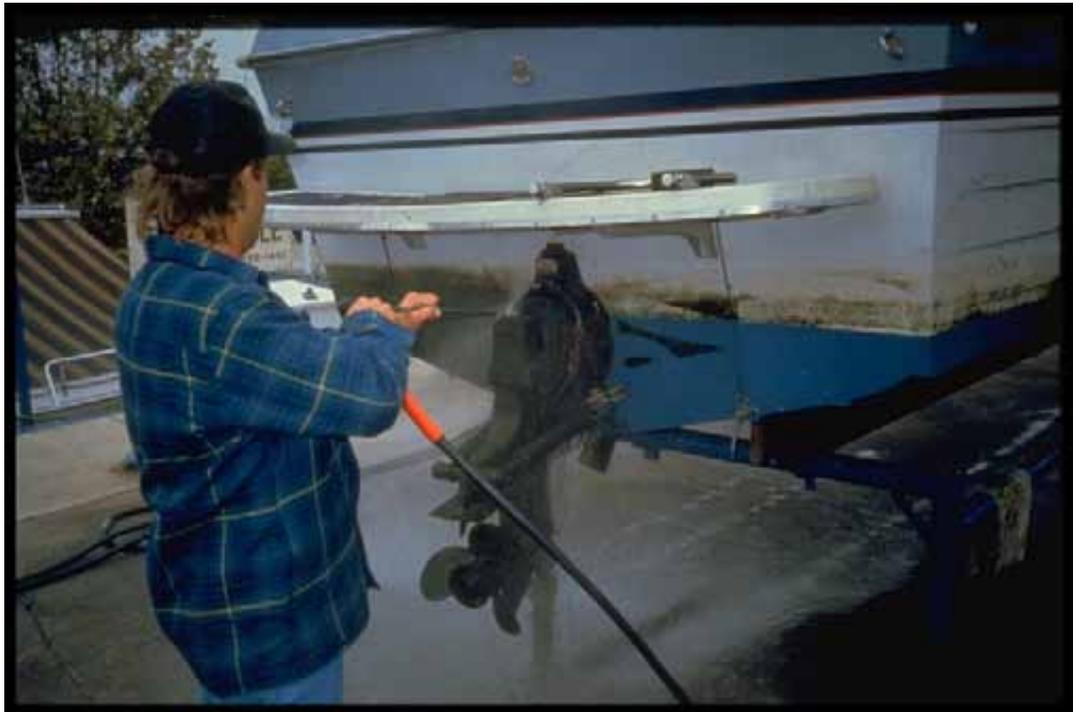
**Figure 21 Power Washing To Remove Mussels (note clean right side compared to left side)**
