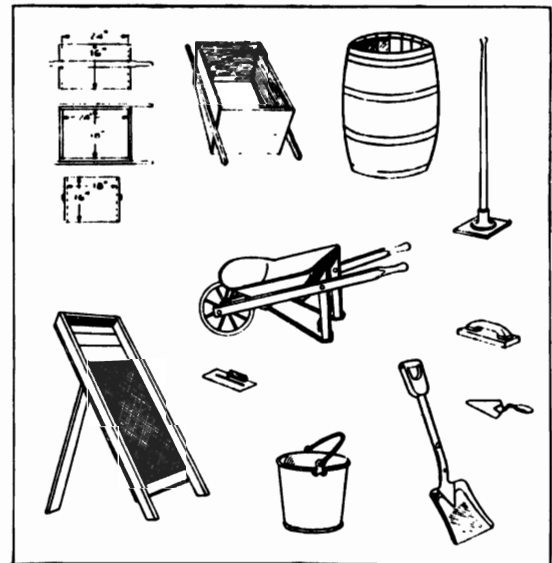
Tools commonly used in farm concrete work.
