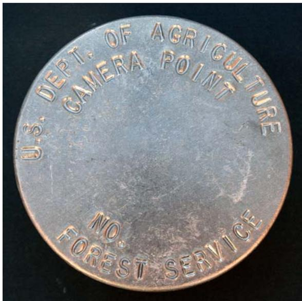
**Figure 2:** Aluminum cap used with the camera point marker described in figure 1. This figure shows the standard wording supplied with the aluminum tap-on camera point cap. It allows space on the bottom half (just above "FOREST SERVICE" and to the right of "NO.") to scribe your actual camera point number in the field. The sharp tip of a nail or another scribing tool can be used to add the camera point designation (e.g., "T-96-1" as shown in exhibits 2 and 4) to this portion of the cap.
