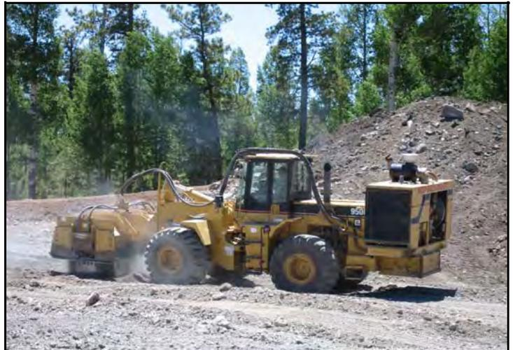
*Mobile trimming unit generates aggregate material in a Forest Service gravel pit*
