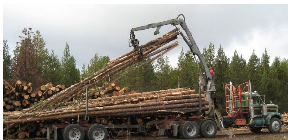
Figure 1: Self-loading log truck with small diameter lodgepole pine logs. Credit: L. Swan
