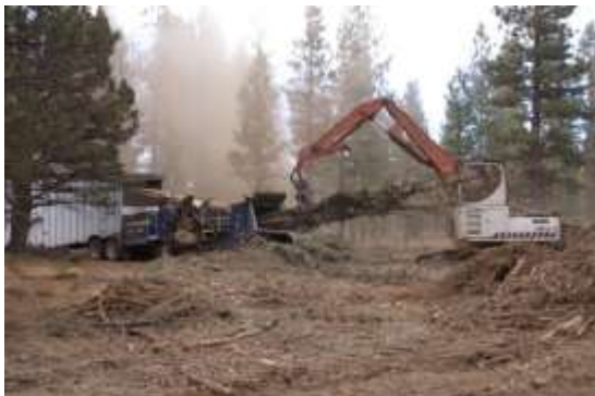
Here loggers feed trees too small to be used as saw logs into the chipper for transport to the biomass facility.
