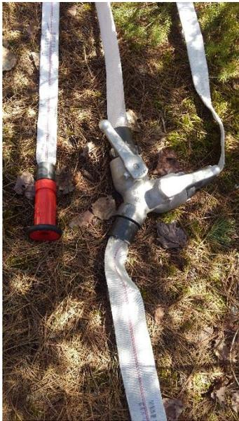
*Y valve and nozzle on hoselay for prescribed fire line holding*
