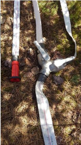
*Y valves with nozzles on a hoselay allow fire managers to control lines on prescribed burns.*
