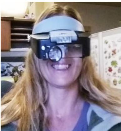
Figure 37. Binocular magnifier that can be used for monitoring adelgid nymphs. Photo by Marie McLaughlin.
