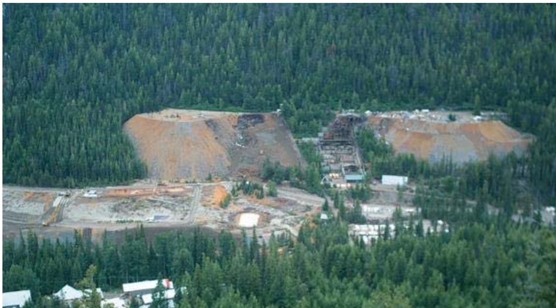
Figure 3. View of the Former Mill Building, Tailings Piles, and Waste Rock Piles.
