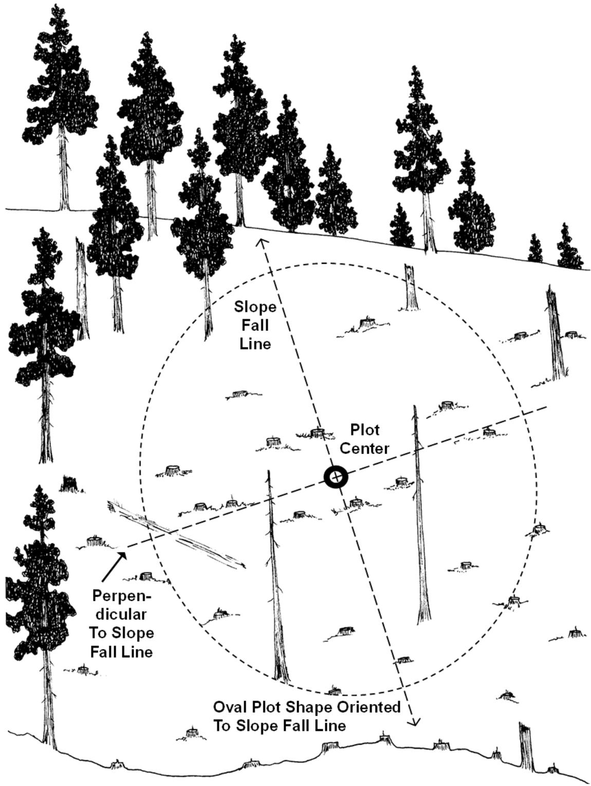
On sloping ground, plots have an oval shape with their long axis parallel to the slope (called 'slope fall line'). Note that a line perpendicular to the slope forms a 'right angle' with the slope fall line. Plots on sloping ground need to have their radius adjusted by using a factor that converts slope distance to what is called horizontal distance.
