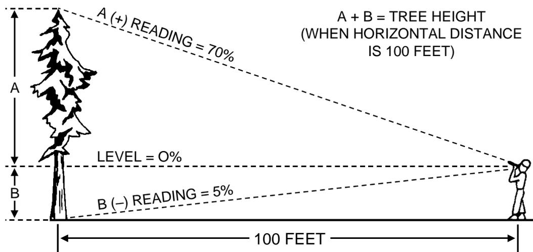
The A (+) readings on a clinometer mean that you are looking up; the B (-) readings mean you are looking down. Level (not up or down) readings are 0 on a clinometer. In our example
