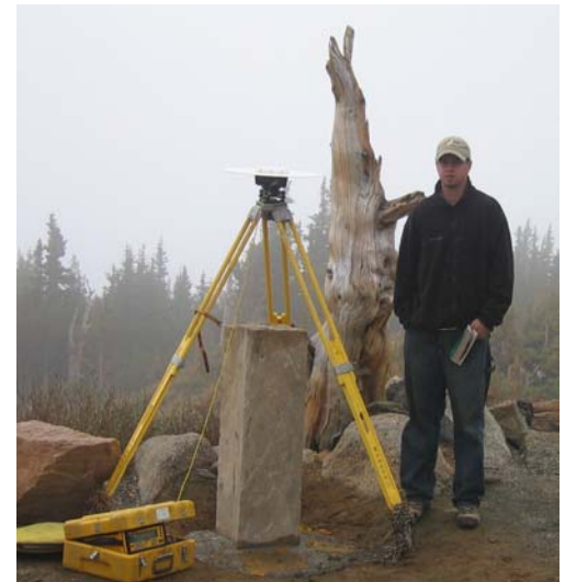
Above: ARP Survey Technician Zach Deitrick establishes that the monument is located at precisely 11,503.94 feet, Latitude: 39° 28' 32.825", Longitude 105° 35' 33.491"
