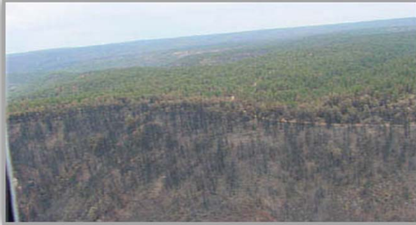
Figure 2 . Aerial view of Rodeo-Chediski area, 2002. The Gatewood Canyon area (foreground) was untreated and suffered extreme fire intensity and stand replacement. The Chuck Box area (background) had been thinned, and fire crews were able to stop the fire at its edge.
