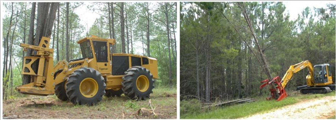
Figure 5 . Images of rubber tired feller buncher and track feller buncher.
