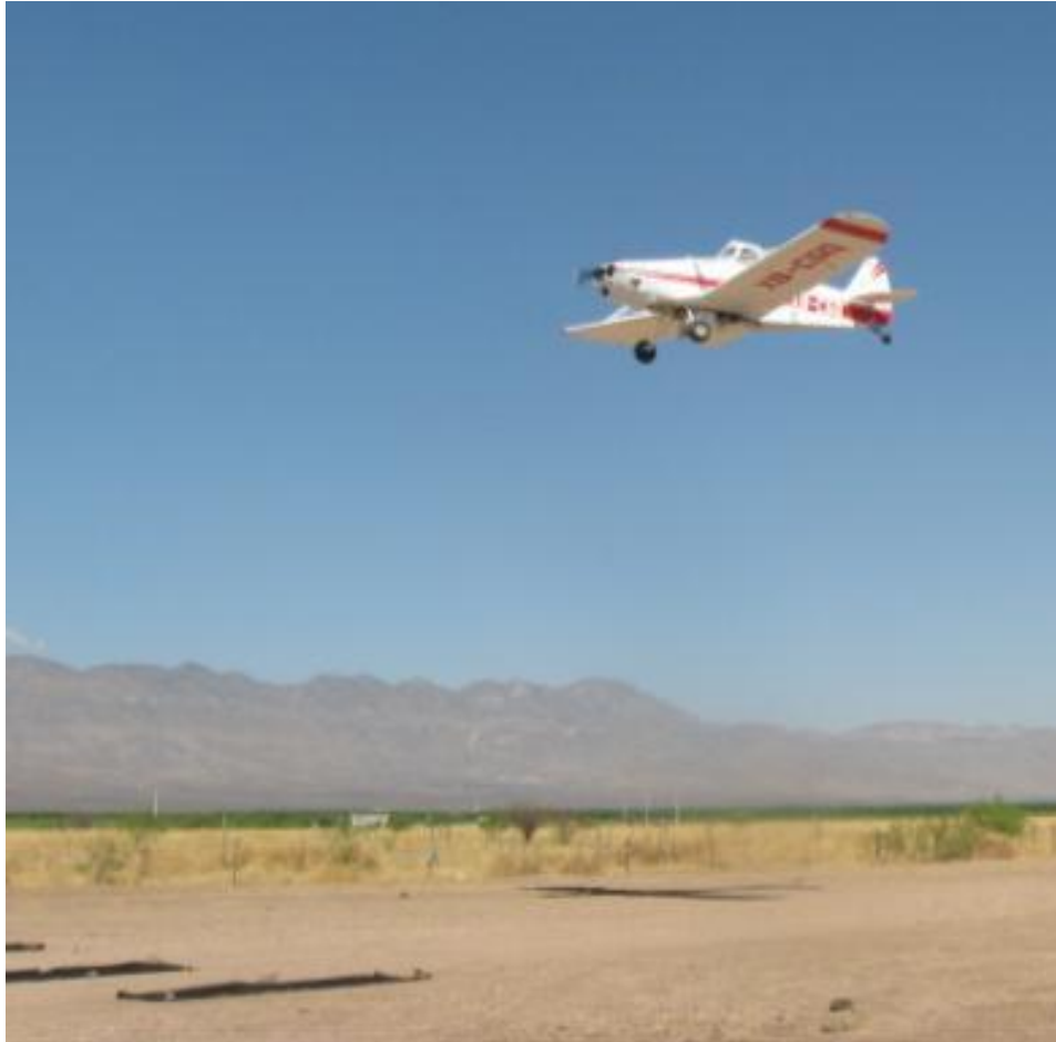
Photo 5: Calibrating the Piper at the Chihuahua airstrip. We laid black weed barrier fabric on the ground so we could see the distribution of flakes.
