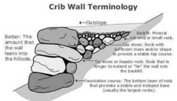
will make the difference in your wall lasting a year or a hundred years. Use smaller angular rocks to fill any gaps as you go. Do not rely on smaller rocks to keep a larger rock in place.
