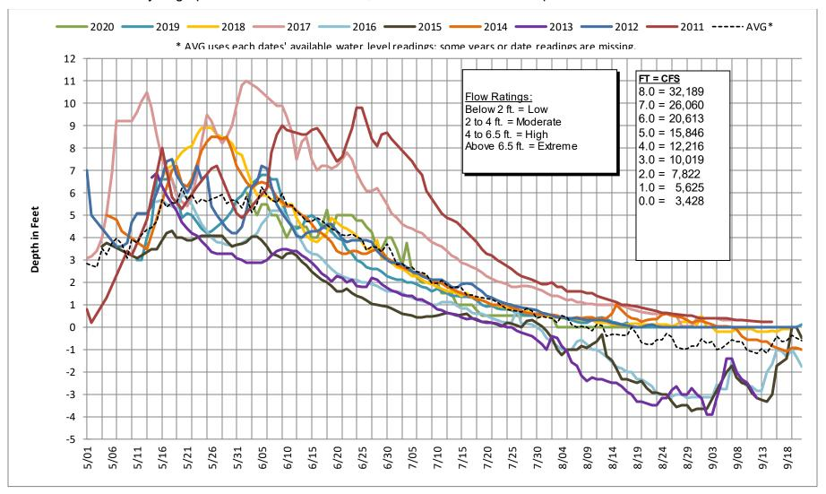
Note: This hydrograph is a very general guide for predicting flows. The lines merely connect depth points which were read on the dates shown. Considerable fluctuation can occur daily, especially on very warm days and after high-intensity rain storms.
