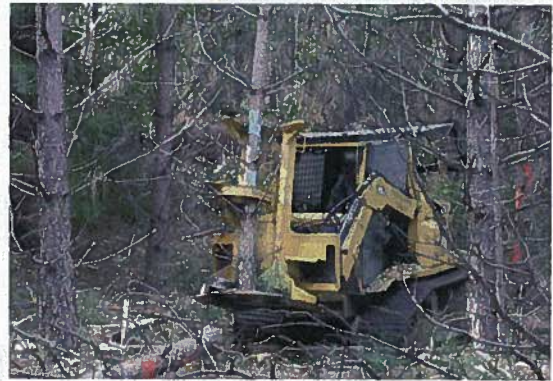
Figure 1. A feller buncher removing small trees that act as fuel ladders and transmit fire into the forest canopy.
