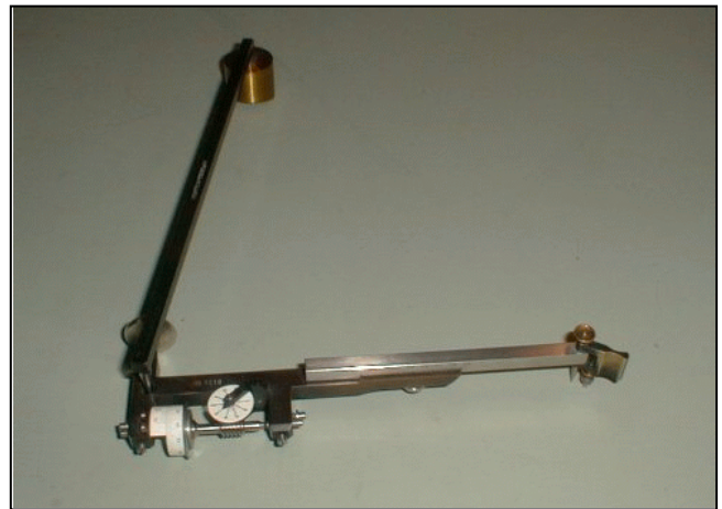
This is a planimeter, a drafting instrument used by surveyors that mechanically calculates the area of a graphically represented planar region (of a map, etc.)
