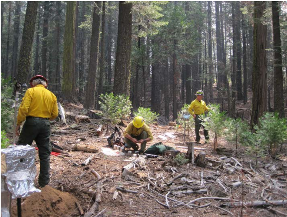
Figure 3: Examples of fire behavior equipment set up at the Willow Fire at plot 2. Viewing diagonally from left to right next to the workers are the heat flux sensor, the thermocouple cans (to be buried to measure spread rate), and in the distance is the video camera box.
