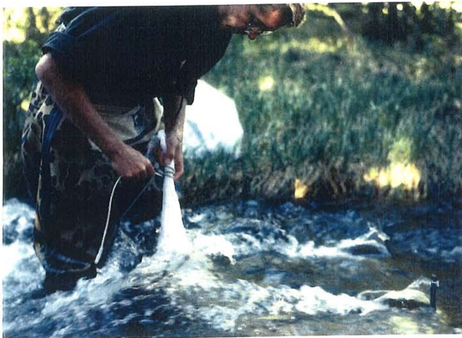
Photo 4: The net is tied shut and put back into the flow for another sampling period.
