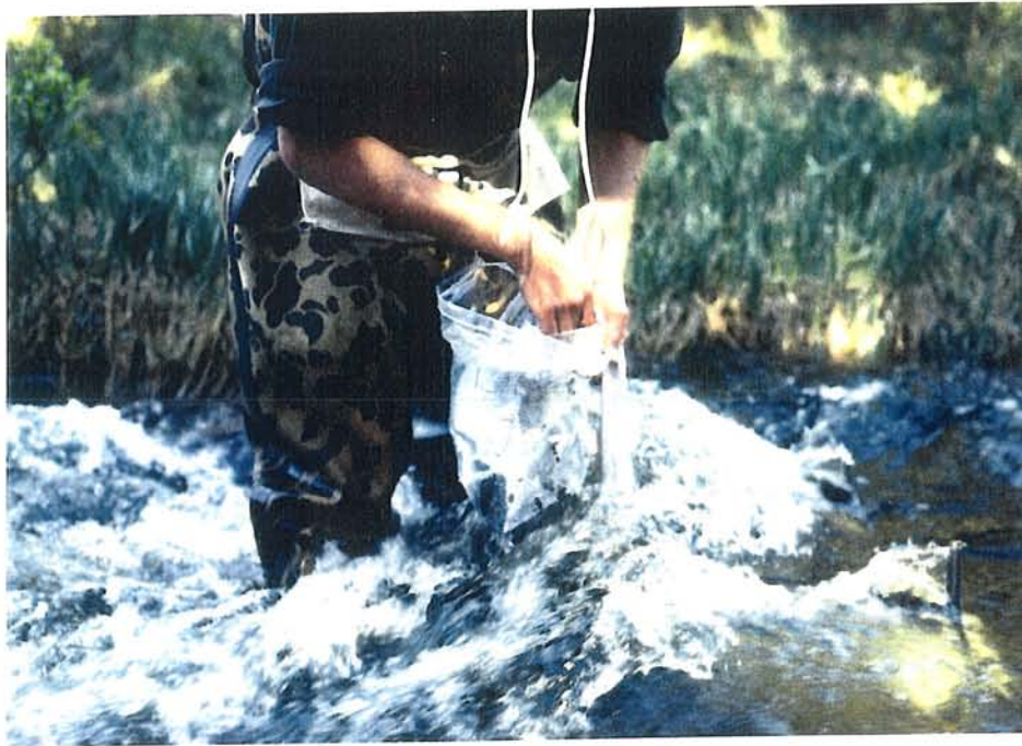
Photo 3: ...and all debris and bedload is shaken into a large ziplock bag
