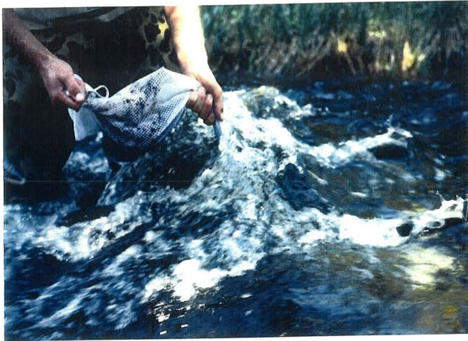
Photo 1: For emptying the sampler, the end of the net is lifted out of the flow. All debris and bedload collected in the sampler are shaken to the end of the net before untying the clothline.
