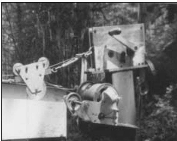
Figure 2. Key components of the cableway. Traveling block, sounding reel, and crank-pulley mechanism. The pulley housing remains on site between measurements, but the sounding reel is removed to deter vandalism.
