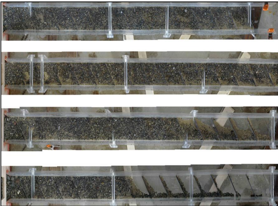
Figure 4-25. A photo showing the sediment accumulation in the high, close-spaced, full-spanning angled baffle culvert model at a slope of 2.0% and flows of 0.06, 0.095, 0.195 and 0.34 cfs, respectively from top to bottom. The view is looking down from above the flume model.
