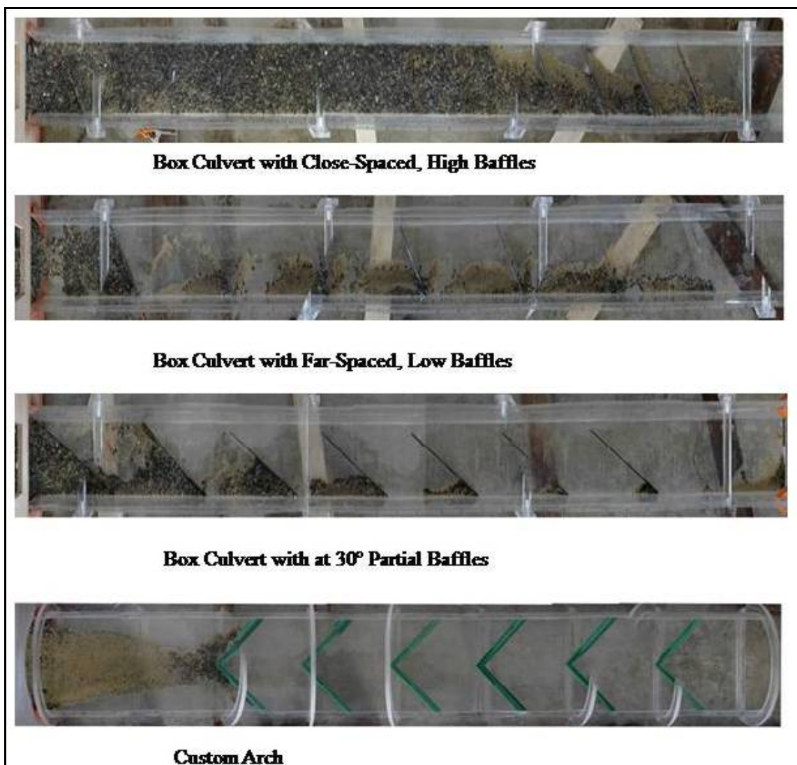
Figure 4-28. Photos comparing sediment accumulation in all culvert models at 2.0% slope and 0.195 cfs flow.
