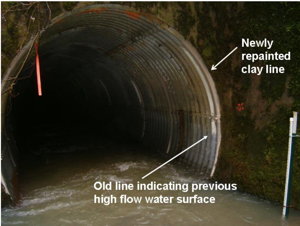
Figure 3-8. Clay line sets at Chadd Creek. New lines are repainted adjacent to the previous line to preserve and compare records.
