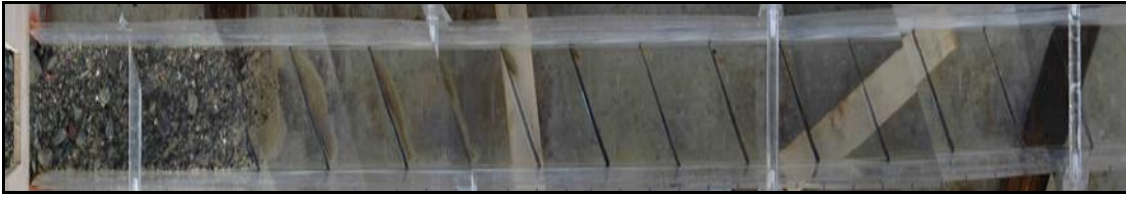
Figure 4-24. A photo showing the sediment accumulation in the high, close-spaced, full-spanning angled baffle culvert model at a slope of 0.5% and a flow of 0.34 cfs. The view is looking down from above the flume model.
