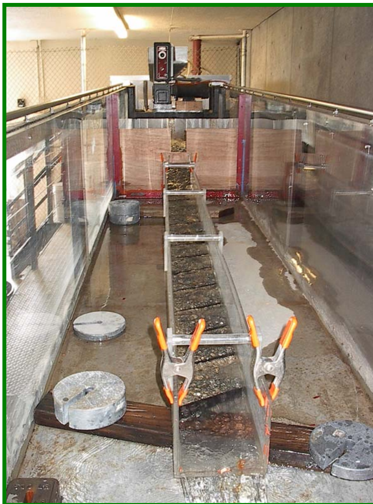
Figure 3-4. Looking upstream at the experimental set-up in the flume for a box culvert.
