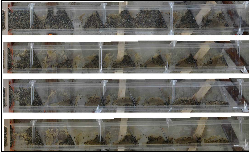
Figure 4-26. A photo showing the sediment accumulation in the low, far-spaced, full-spanning angled baffle culvert model at a slope of 2.0% and flows of 0.06, 0.095, 0.195 and 0.34 cfs, respectively, from top to bottom. The view is looking down from above the flume model.
