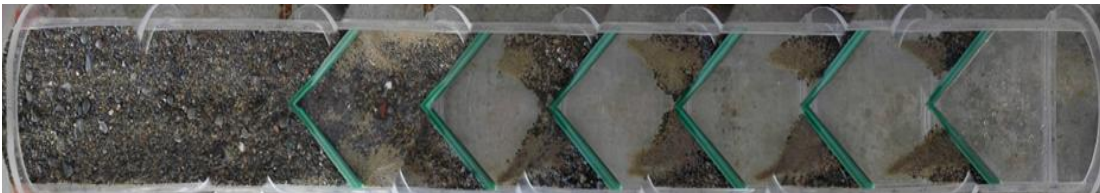
Figure 5-15. Observed sediment accumulation in the custom arch culvert with vortex weirs at the 4.0% slope and highest armoring flow of 0.34 cfs. The flow direction is from the left (inlet) to right (outlet).
